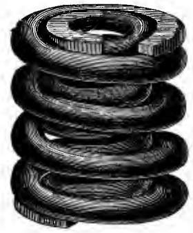
Fig. 5247. ROUND-BAR DOUBLE-COIL BUFFER-SPRING. (Capacity, 16,000 to 18,000 lbs.)
